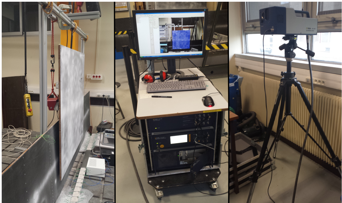
Figure 6.2: Testbed realized to measure the displacement field of the sandwich panels.
