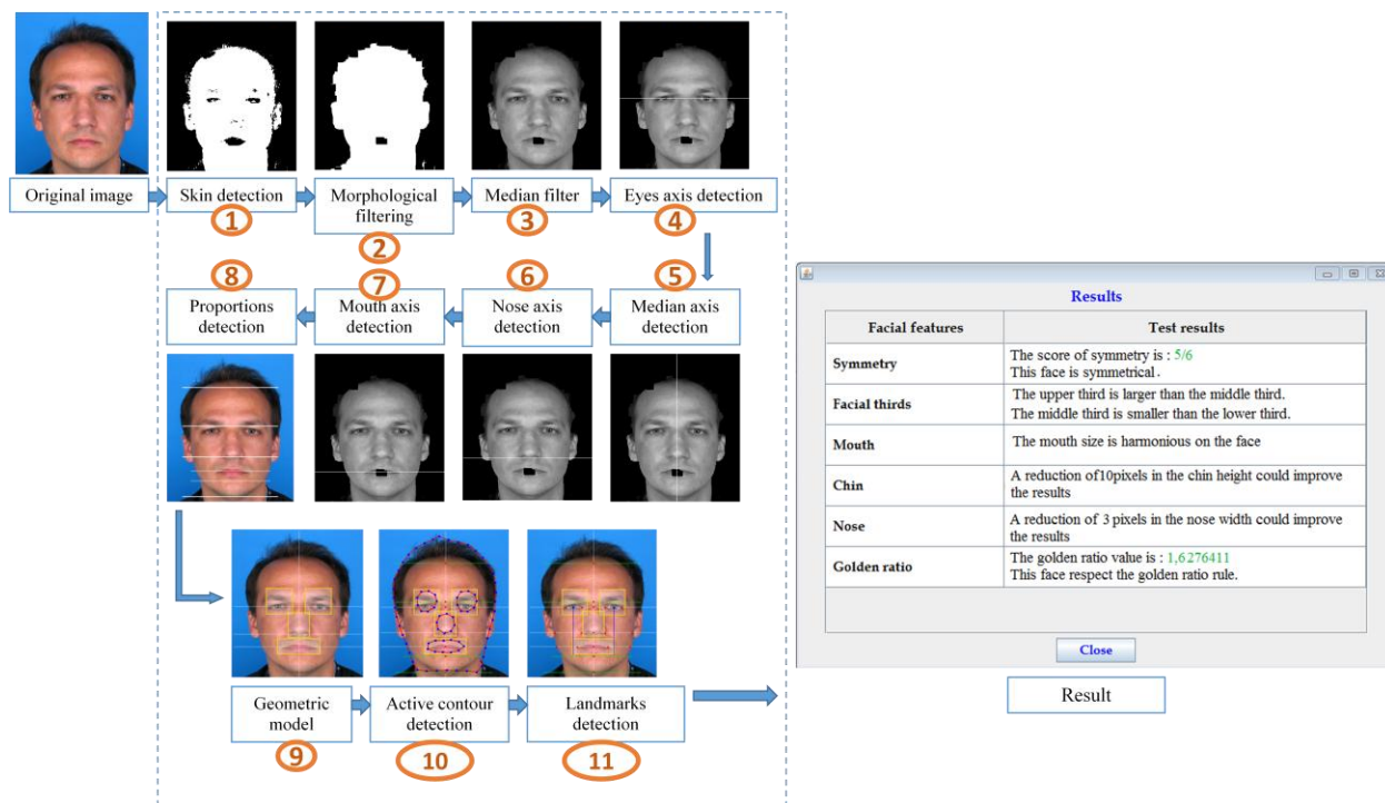
Figure 2.1: Global architecture of the proposed method to analyze the aesthetic quality of faces.
