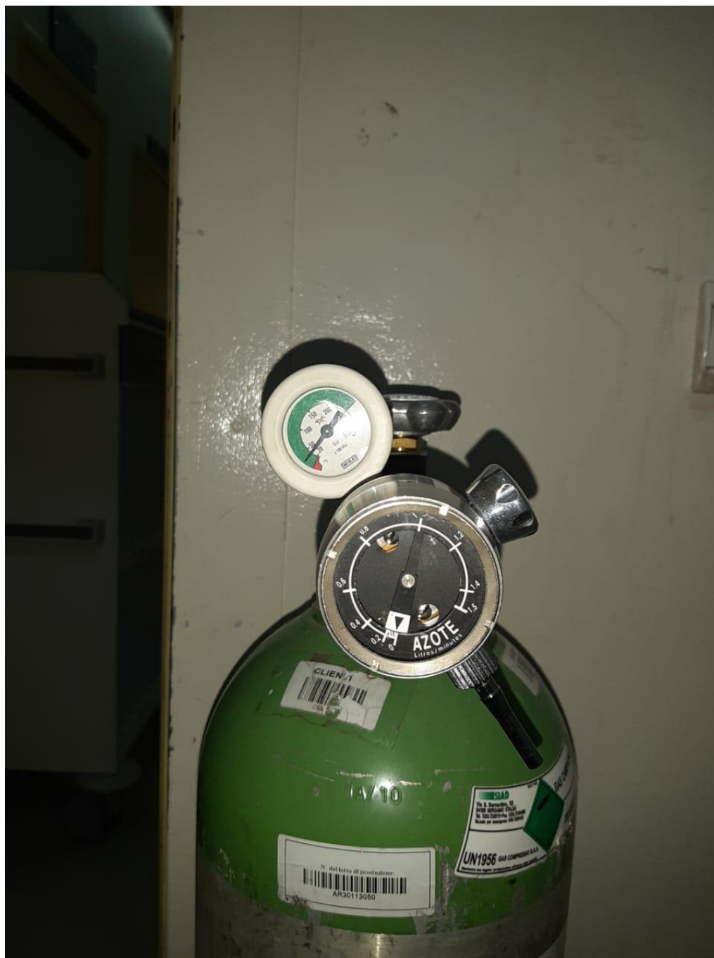
IMAGE 1. Showing the manometer used for delivering iNO dose from 0.2 to 1.5 liter per minute. University hospital center HASSAN II PICU.
