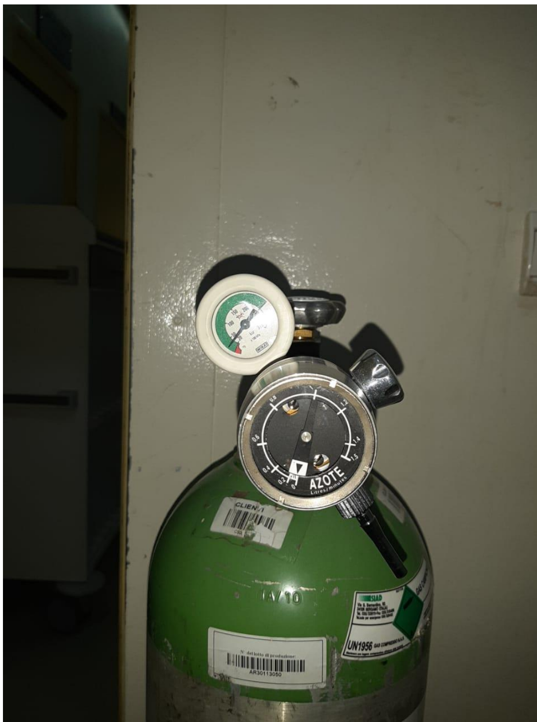
IMAGE 5. Showing the manometer used for delivering iNO dose from 0.2 to 1.5 liter per minute. University hospital center HASSAN II PICU.
