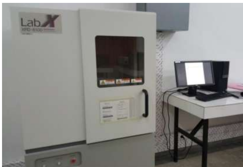
Figure 2.13: Shimadzu 6100 diffractometer available at the Faculty of Science of Rabat
