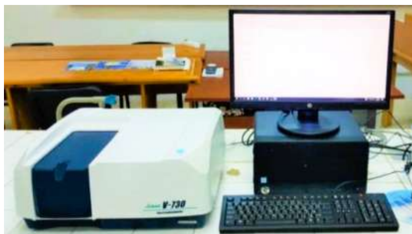
Figure 2.15: UV-Vis spectrophotometer (Jasco model V-730 available at the LMNE Laboratory
