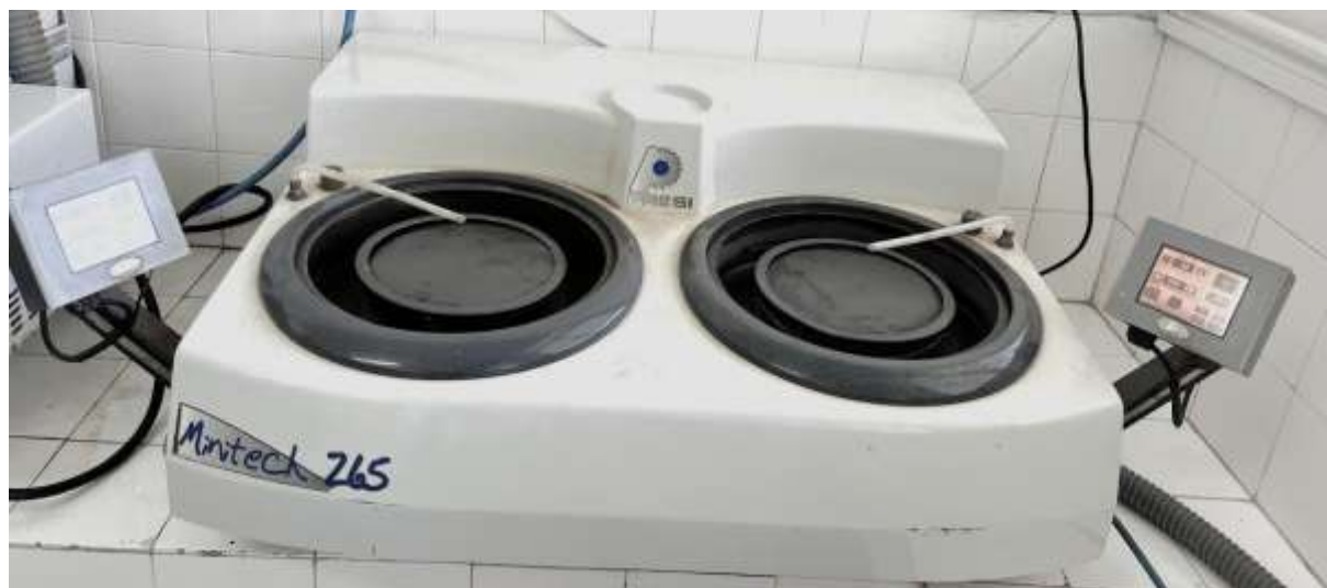
Figure 2.1: Variable speed 20- 700tr/min manual Polishing machine available at LMNE Laboratory
