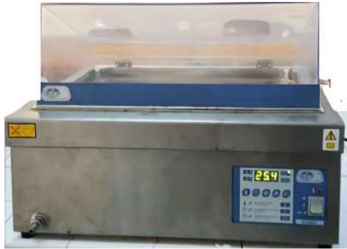
Figure 2.2: Thermostatically controlled water bath used in gravimetric studies at the LMNE Laboratory
