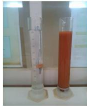
Figure II-78: Test de sédimentation
