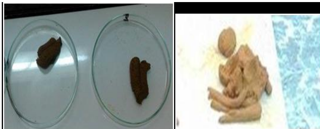
Figure II-33: Test de ressuage
