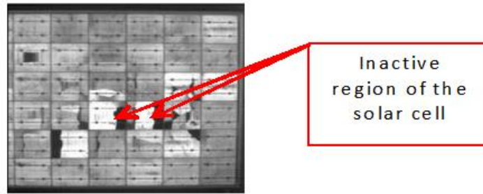
Fig.1.12. EL of a PV module with occurring Broken cells [9]
