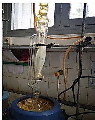
Figure.II. 9: The hydroalcoholic extraction setup of coffee grounds using the Soxhlet process and rotavapor.
