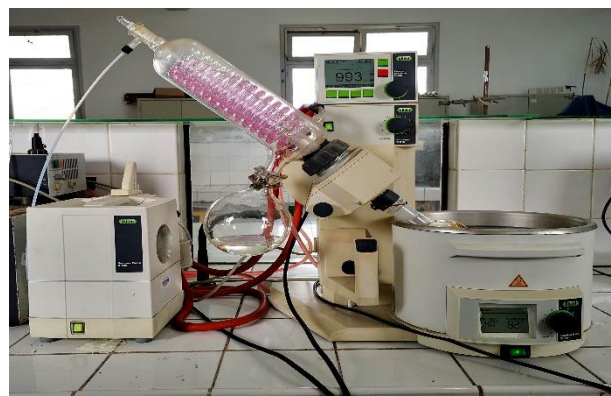
Figure.II. 9: The hydroalcoholic extraction setup of coffee grounds using the Soxhlet process and rotavapor.
