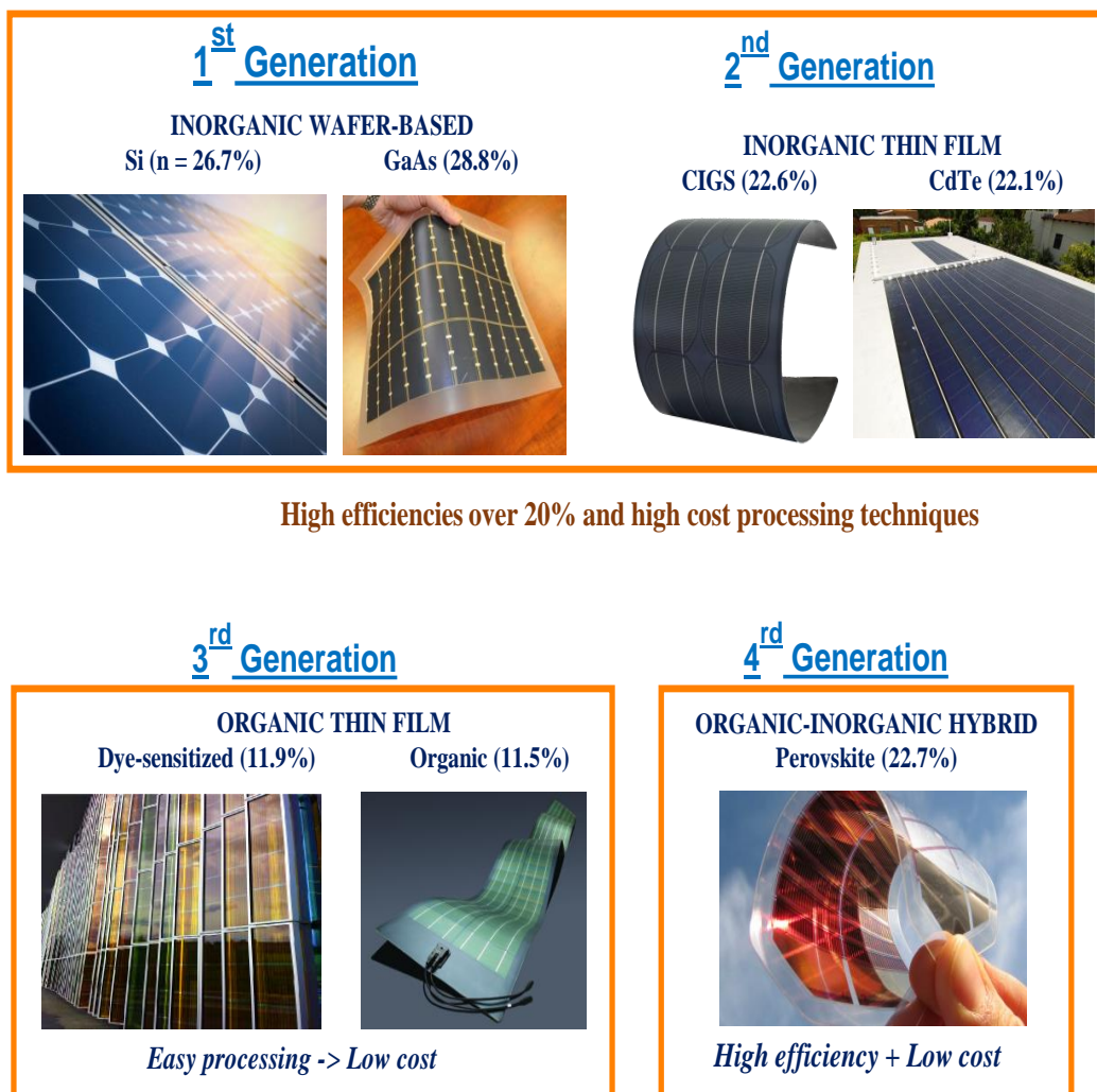
Figure 1.2: Generation solar cell technologies .
