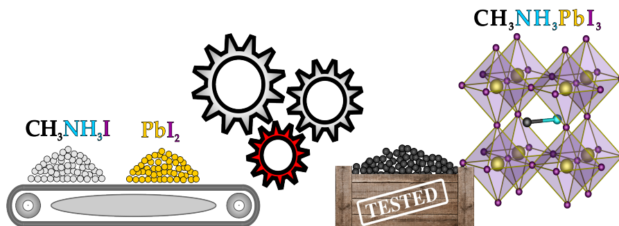
Figure 1.4: Methylammonium Lead Iodide \text{CH}_3\text{NH}_3\text{PbI}_3 is an organometal halide perovskite system that is used as an absorber in solar cells. co-evaporation of Methylammonium Iodide ( \text{CH}_3\text{NH}_3\text{I} ) and Lead Iodide ( \text{PbI}_2 ) require treatment of the resulting \text{CH}_3\text{NH}_3\text{PbI}_3 thin film to catalyze the reaction between \text{CH}_3\text{NH}_3\text{I} and \text{PbI}_2 and create a pure perovskite phase.
