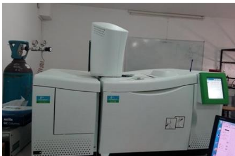
Figure III- 4 : Appareil GC /MS Clarus 680.
