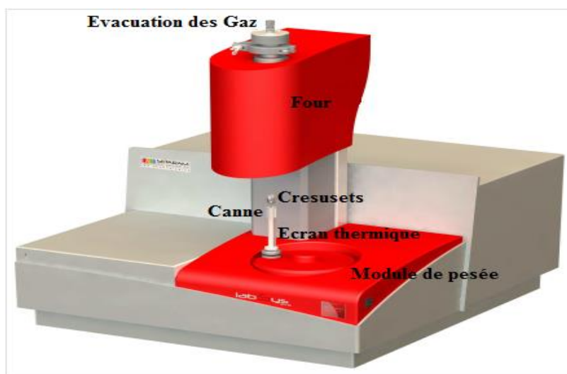
Figure III- 7 : Appareil thermique LABSYS EVO (SETARAM).
