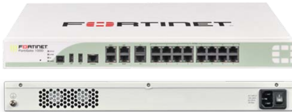
Figure 6 : Serveur Firewall Fortigate.
