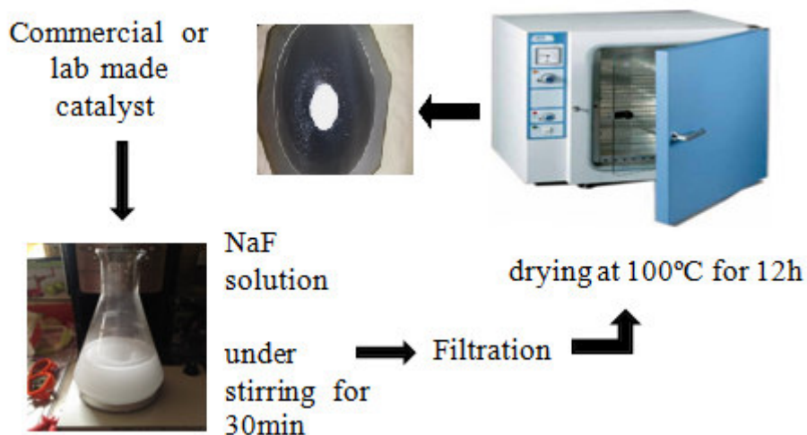
Figure III.3 : The experimental process of doping the catalysts by fluorine (F-MO x )
