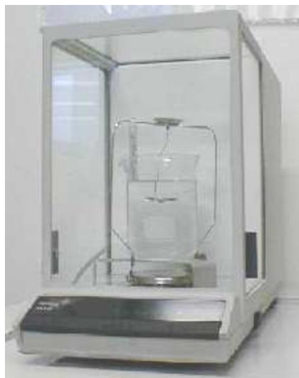
Figure II. 1. Experimental device of the Archimedes method.
