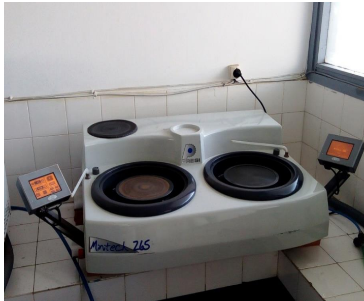
Figure II. 15. Manual polishing machine with variable speed from 100 to 500 rpm.
