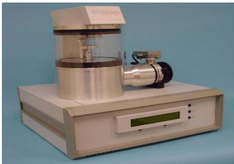
Figure V.1: K575X turbo Sputter Coater used for Pt NPs deposition
