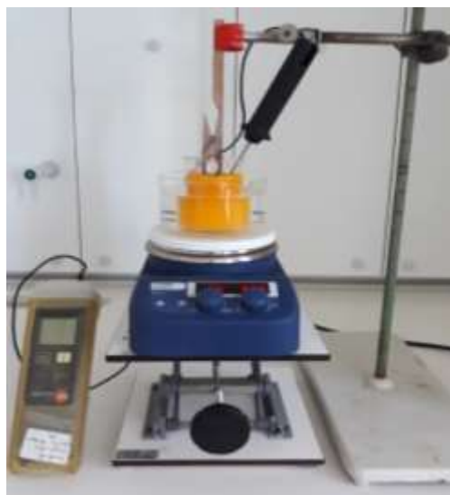
Figure II.7 Montage de la technique CBD.
