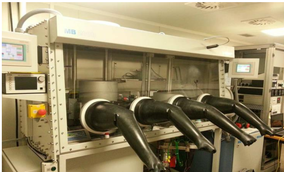
Figure 7.8: Glovebox MB200B from MBraun with thermal evaporator, solar simulator and EQE techniques inside chamber.
