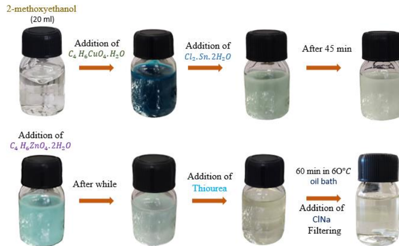
Figure 5. 1: Protocol used to prepare the CZTS Sol-gel solution.
