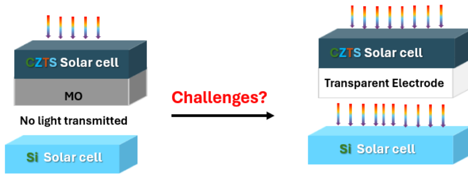
Figure.5. The challenges to develop tandem configuration using CZTS as top solar cells
