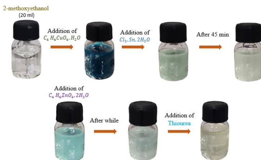
Figure 4. 1: Protocol 1 used to prepare the CZTS solution.
