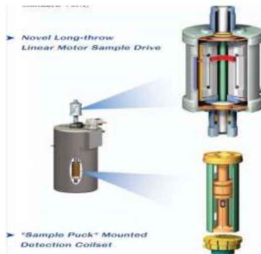
Figure 33. Schematic of VSM magnetometer
