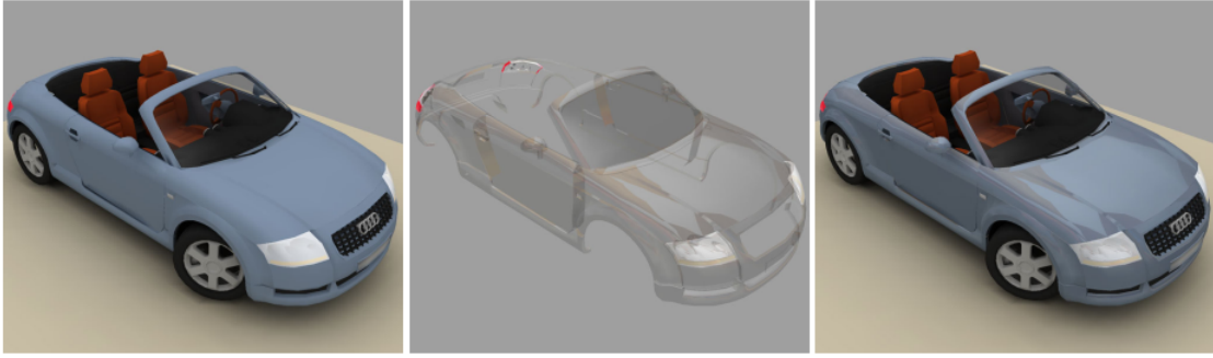
Figure 2.5 Example of spherical harmonic lighting on a 3D car object (Green, 2003).
