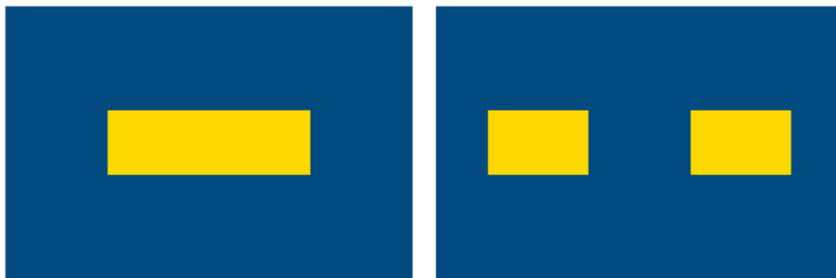
Figure 1.6 A simple example of two different images whose histograms and color coherence vectors are almost similar and color correlograms are different (Huang et al., 1997).
