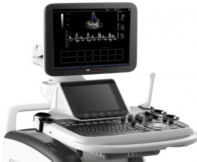
Figure 16 : appareil doppler transcrânien duplex.
