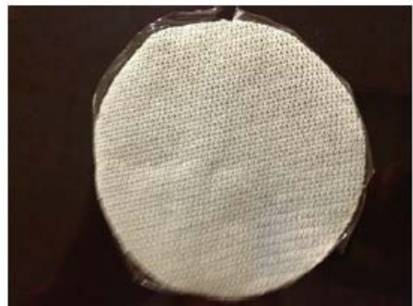
Multifilamented polyester with a microporous absorbable collagen barrier
