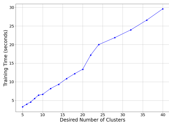
Figure 2.9: Training time across desired number of clusters within our experimental InSDN dataset
