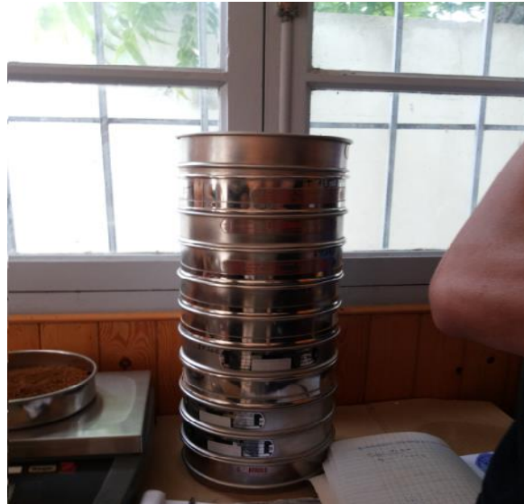
FIGURE 30. THE GRAIN SIZE DISTRIBUTION ANALYSIS.
