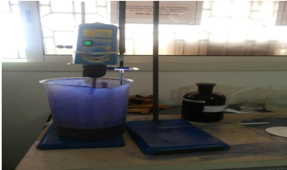
FIGURE 37. ELECTRIC MIXER USED FOR STIRRING THE SOIL-METHYLENE BLUE SOLUTION.
