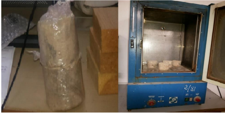
FIGURE 49. DRYING OF TEST SAMPLES.
