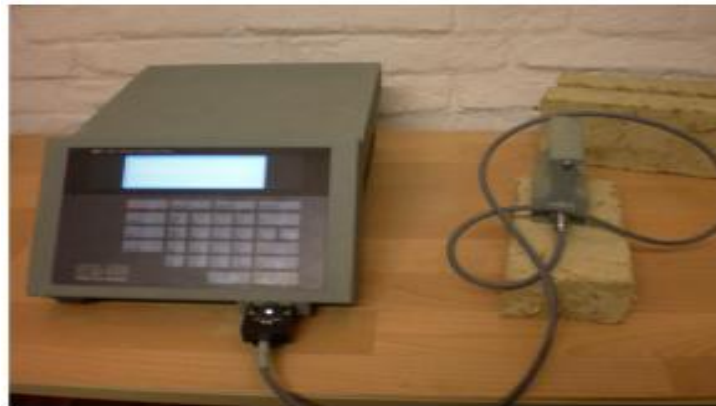
FIGURE 20. THERMAL CONDUCTIVITY INSTRUMENT (THE QTM-500 -METER).
