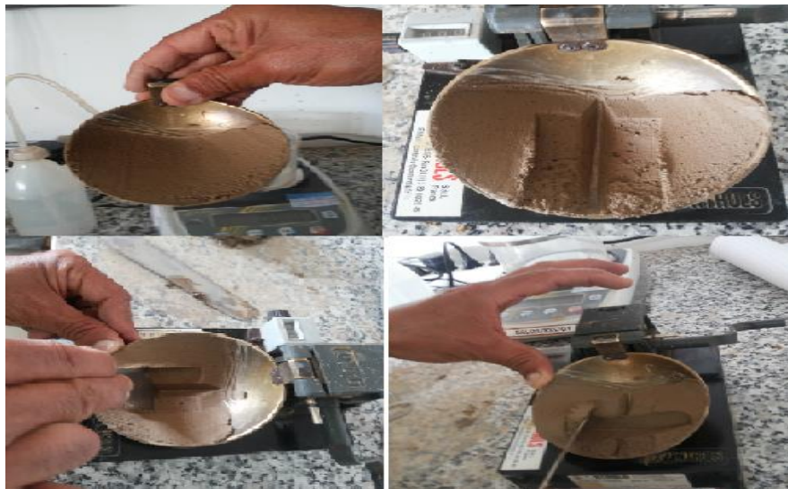
FIGURE 33. LIQUID LIMIT TEST PROCEDURE OF SOIL FEZ.
