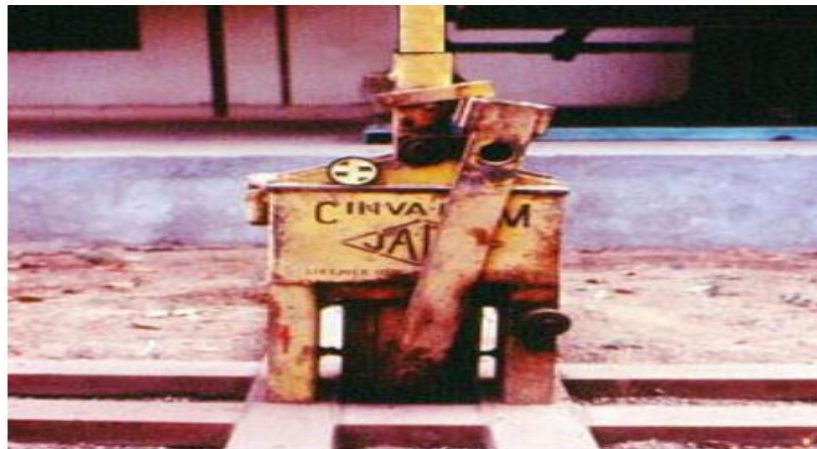
FIGURE 27. ORIGINAL CINVA RAM PRESS [57].
