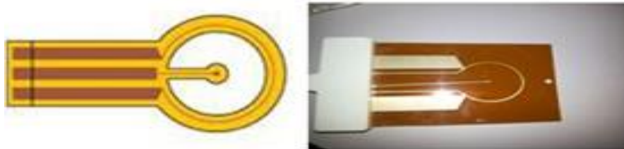
Figure1. Hot Ring sensor
