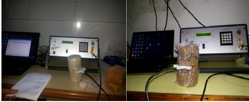
FIGURE 50. THERMAL TESTS OF THE SAMPLES CEBS.
