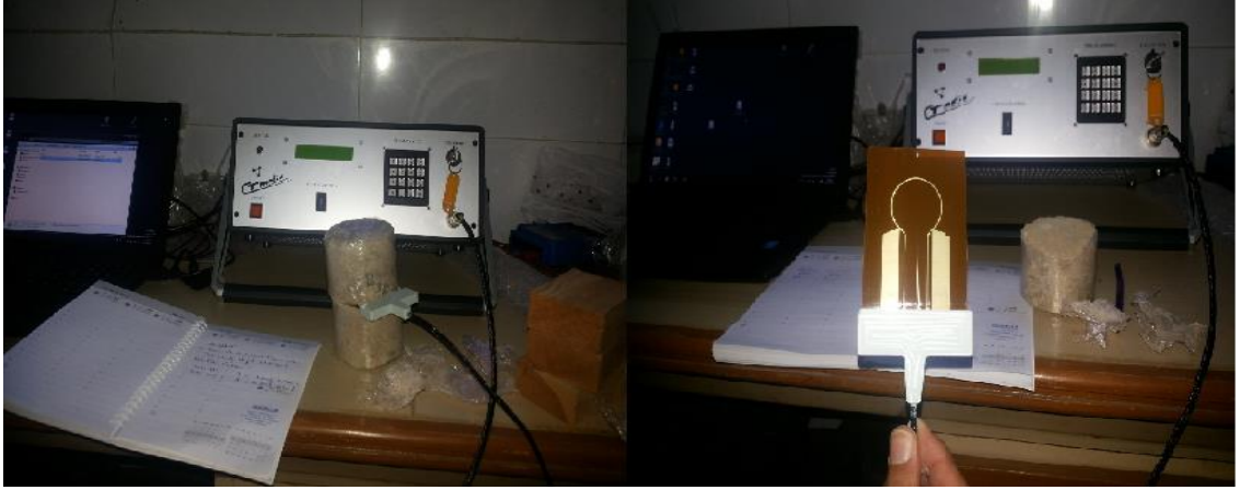
FIGURE 48. THERMAL CONDUCTIVITY MEASUREMENTS BY HOT RING METHOD.
