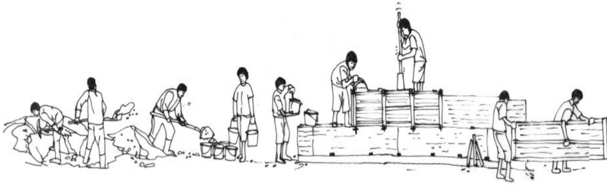
FIGURE 5. RAMMED EARTH BUILDING TECHNIQUES BY EARTH MATERIAL [25].
