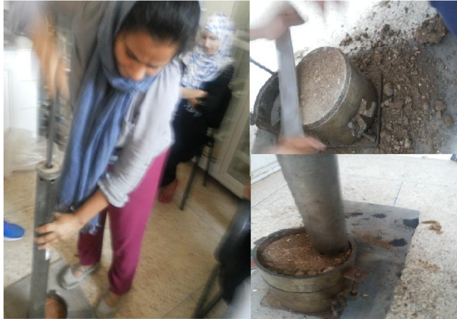
FIGURE 39. PROCTOR SOIL OF FEZ COMPACTION TEST.
