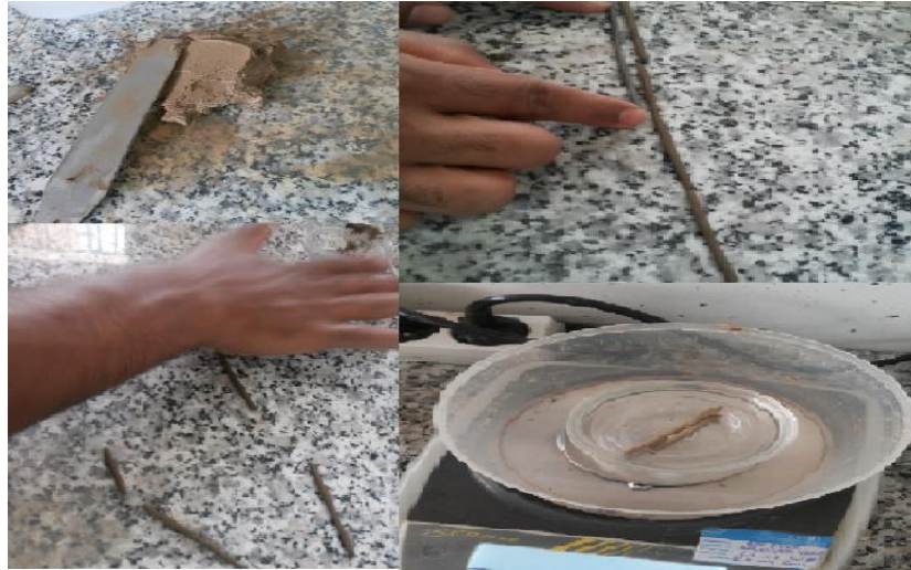
FIGURE 34. PLASTIC LIMIT TEST PROCEDURE OF SOIL FEZ.
