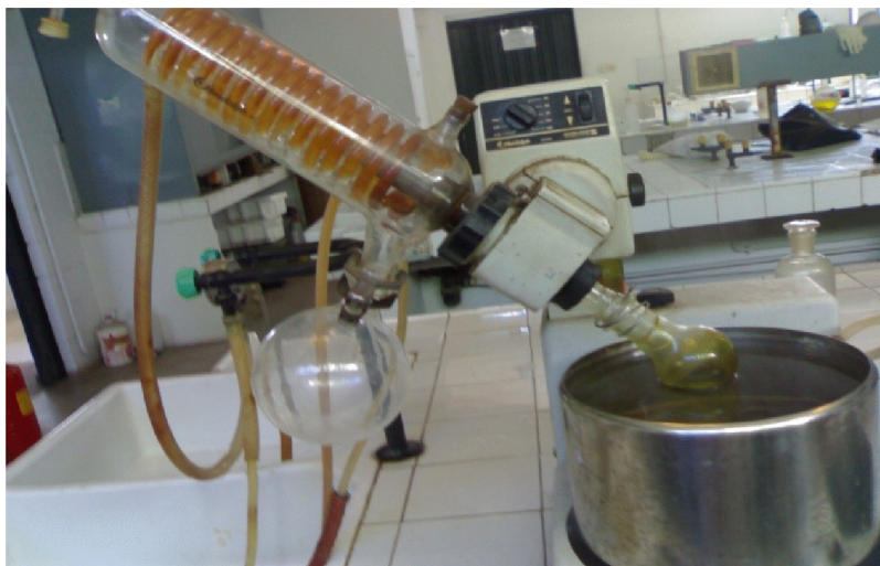
Figure 22 : Evaporation du solvant
