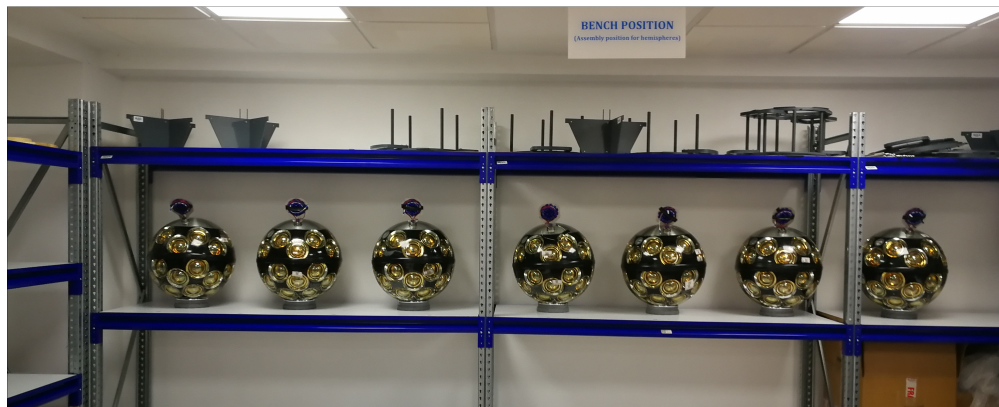
FIGURE 6.37: The first set of 7 DOMs integrated in the Rabat site after successfully passing the acceptance test.
