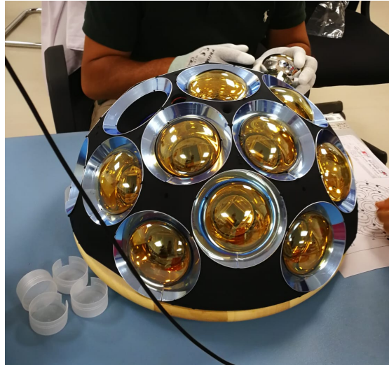
FIGURE 6.21: Bottom PMT support structure being integrated with PMTs and reflector rings.
