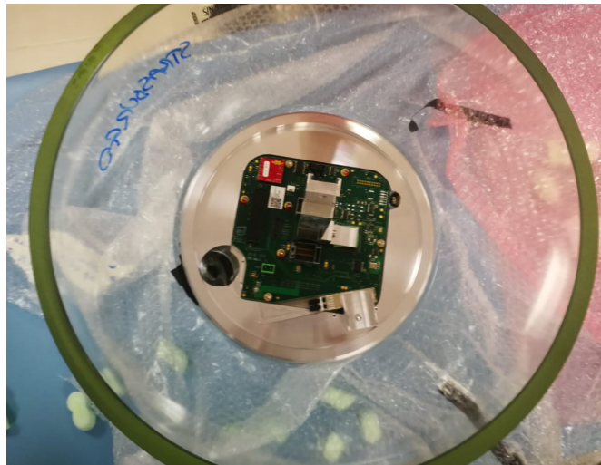
FIGURE 6.25: Top Glass hemisphere after the integration of the cooling mushroom and the electronics.
