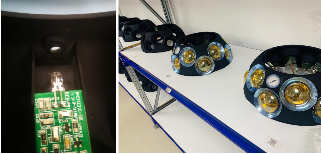
FIGURE 6.29: Left: The led nano-beacon being inserted in its sliding place on the top support structure. Right: The top support structure after the installation of PMTs, pressure gauge and the nano-beacon from the inside.
