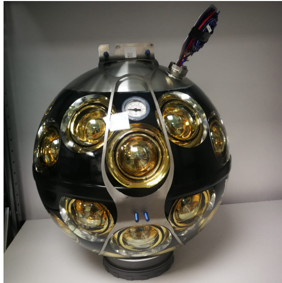
FIGURE 6.38: One of the DOMs assembled in the Rabat site with the collar, ready for shipment.
