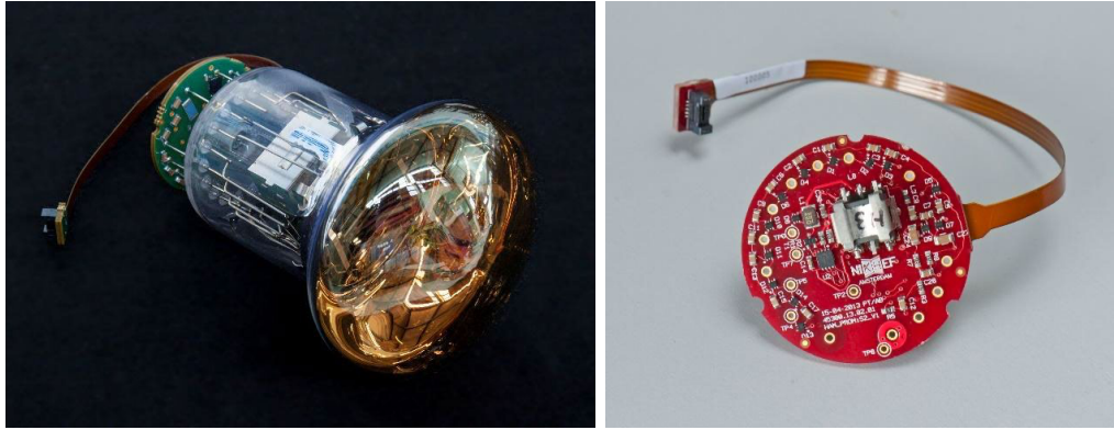
FIGURE 6.12: A Hamamatsu R12199-02 photomultiplier tube with base attached in the left. A photomultiplier base on the right, taken from [100].
