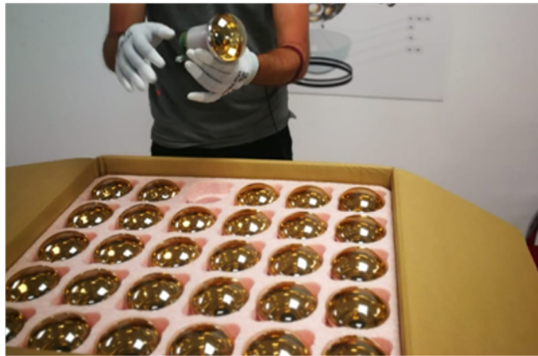
FIGURE 6.13: One of the boxes of PMTs received in the Rabat site, it is advisable to wear anti-ESD gloves while handling the PMTs.
