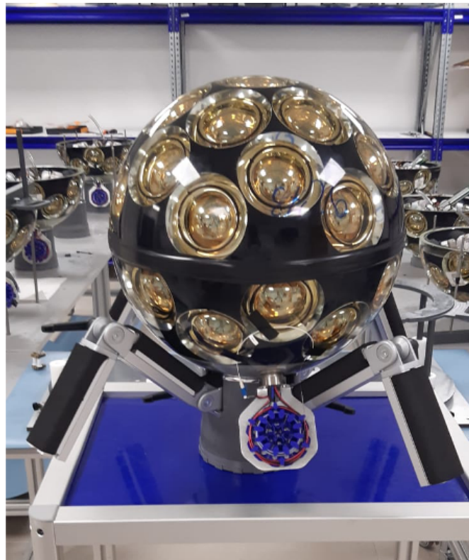
FIGURE 6.6: The first DOM integrated in the Rabat DOM integration site.
