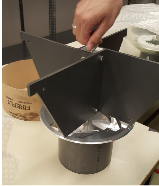
FIGURE 6.23: Cooling mushroom alignment tool, picture taken during the training in Athens DOM integration site.
