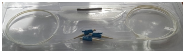
FIGURE 6.18: Add-and-Drop filter, combines the signal coming from 2 optical fibers into one.
