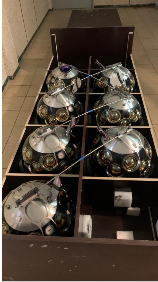
FIGURE 6.8: The first set of 7 DOMs integrated in the Rabat DOM integration site, inserted in the transportation crate and ready to be sent to a DU integration site.
