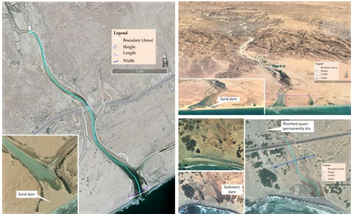
Figure VI. 3: Measuring geometric descriptors in the stream terminal section: three examples of estuarine configuration, in wet and dry conditions.
