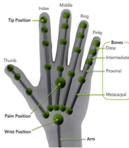
Figure 3-48: Palm and Tip Positions given by the leap motion controller.
