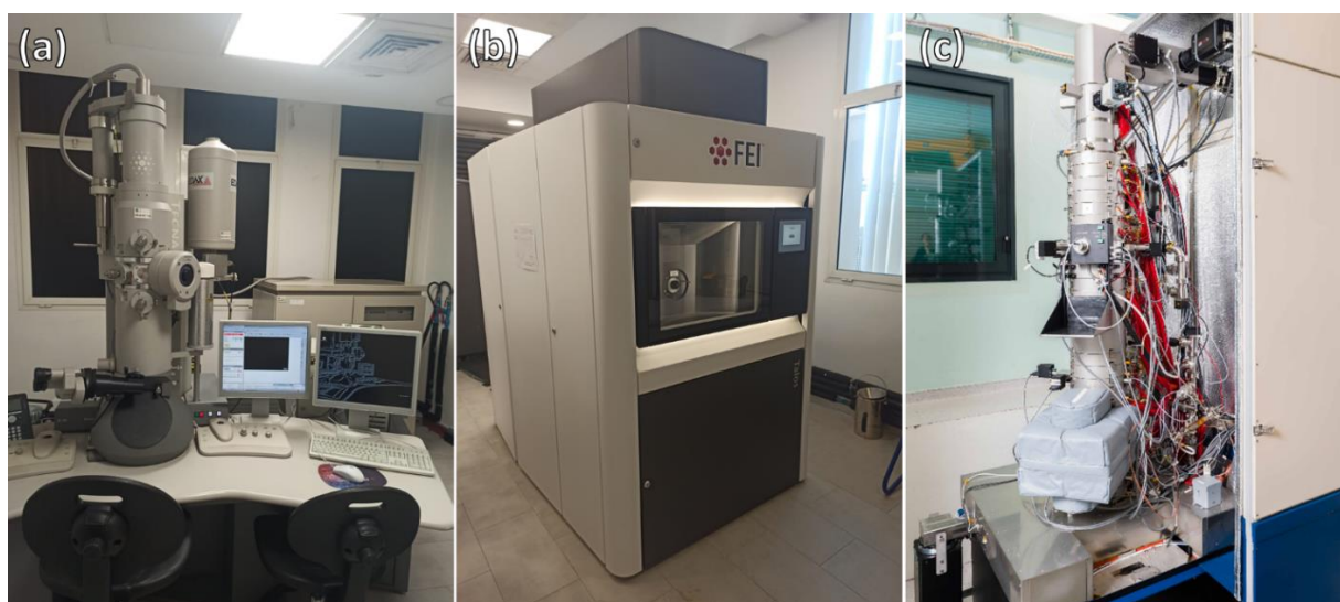
Figure 12 Transmission Electron Microscopes (a) Tecnai G 2 Twin (UATRS-CNRST) (b) FEI Talos 200X S/TEM (UATRS-CNRST) (c) Nion Hermes-S200 (LPS-CNRS) used in our work.
