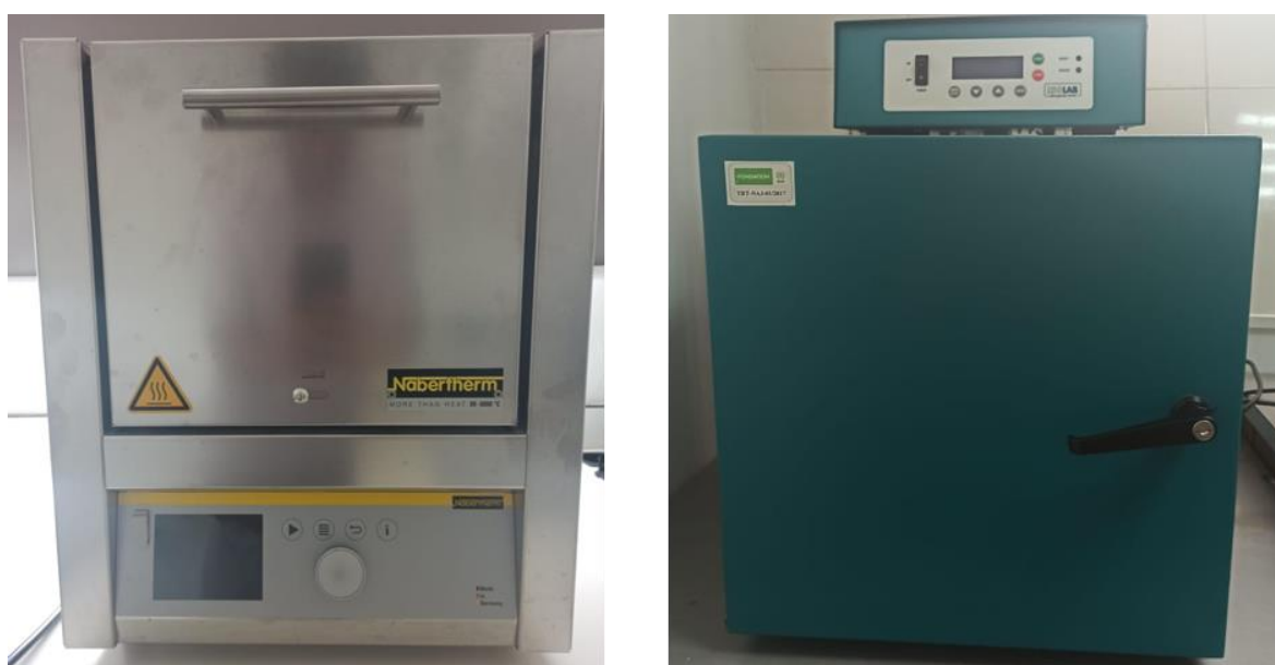
Figure 22. Nabertherm oven used for heat-treatment.
