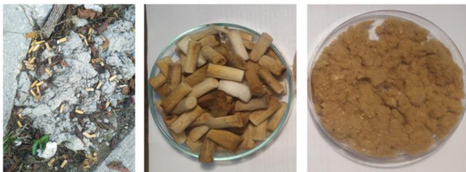
Figure 5-2. Visual aspect of (from the left) the discarded cigarette butts, acetate cellulose fibers separated from the outer paper, and the crushed CAFs.
