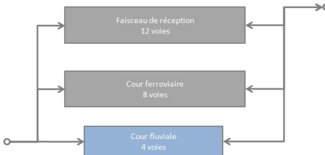
Figure III.5 – Architecture de TMM du Havre
