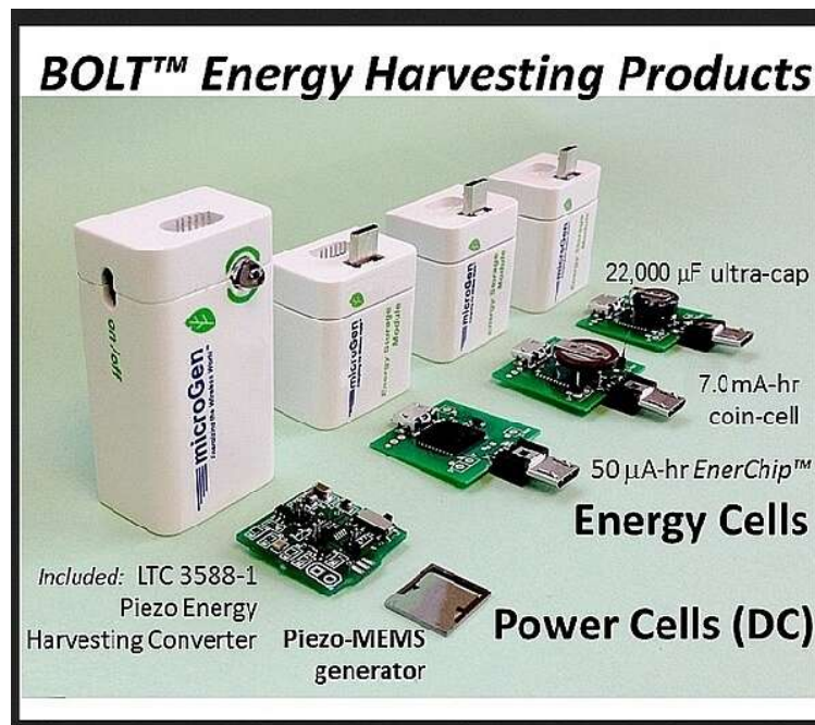
Figure 3.17: From left to right - (1) BOLT™ Power Cell; (2) piezo-MEMS energy harvesting generator or MPG; (3) ESM-B1 using 50 \mu A.hr solid state battery (Cymbet Corp); (4) ESM-B2 using 7.0 mA.hr rechargeable coin cell; (5) ESM-C using 22 mF ultra-Capacitor. Source : Micogen
