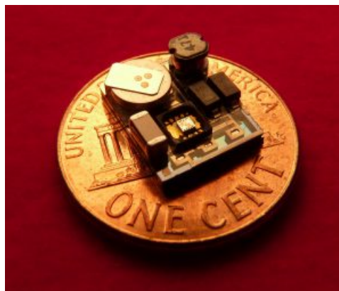
Figure 3.18: Piezoelectric device developed in 2011 at Michigan university. The active part of the harvester occupies a volume 27 mm^3 and the obtained power is 200 \mu W at 1.85V . Source : Michigan University
