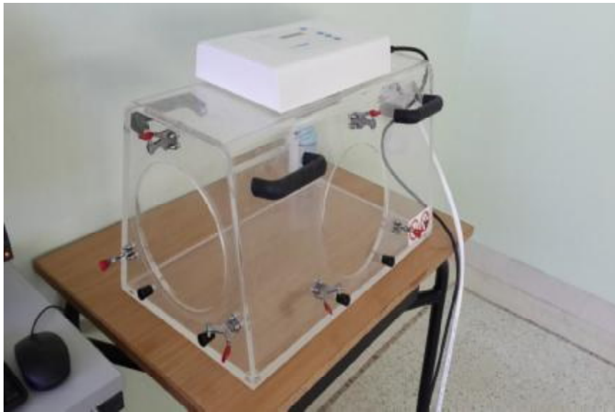
Figure 3: chambre monoplace hyperbare topique
