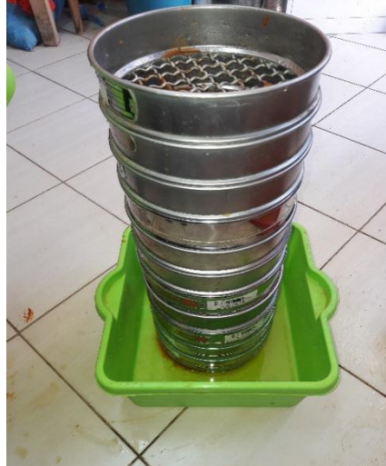
Figure 2. 12: Technique de Tamisage.
