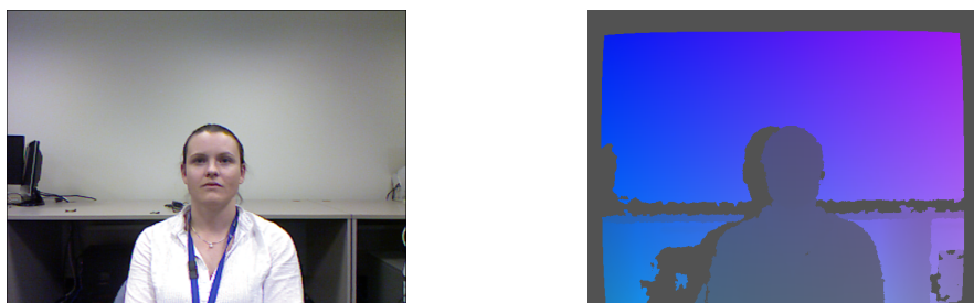
FIGURE 4.2: An rgb image and its depth map acquired from the Kinect sensor
