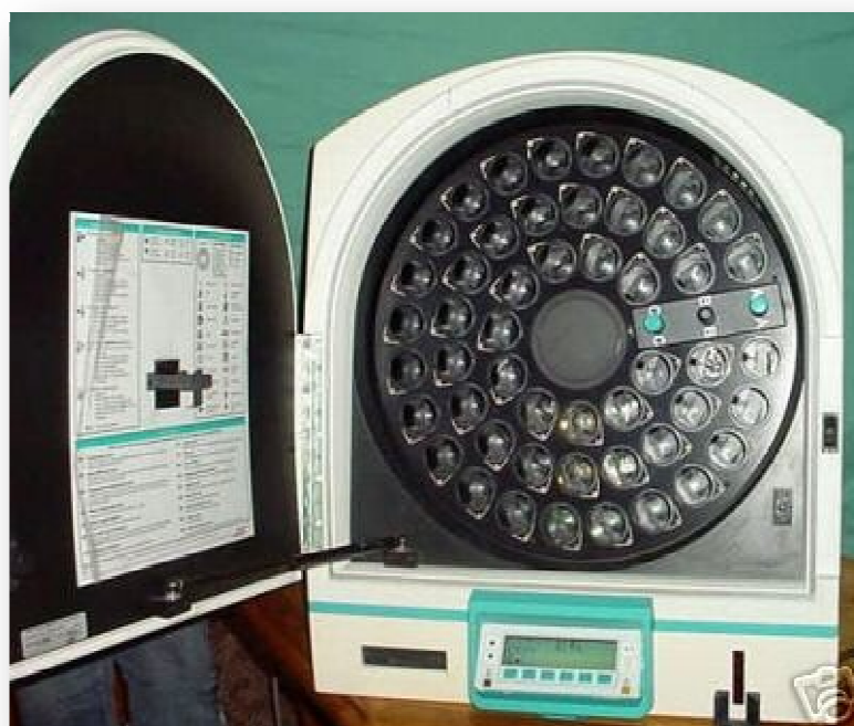
Figure 3b : Automate BACTEC 9050®
