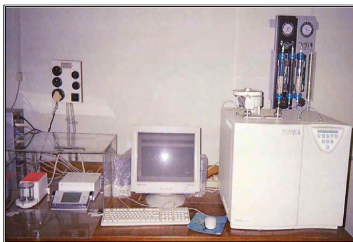
Fig. IV.3: Key components of CHNS are autosampler, combustion reactors, chromatographic column, and T.C.D. detector.
