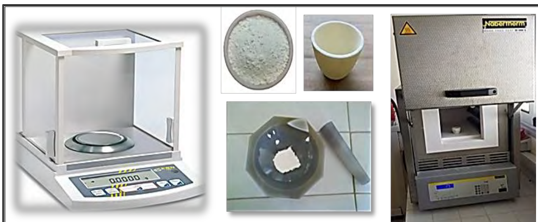
Fig.1: Appliances of the laboratory used in solid-state reactions. Analytical balance sensitivity 0.1mg, example for a sample of lacunar apatite, alumina crucibles, agate mortar, and oven NABERTHERM with and compact muffle.
