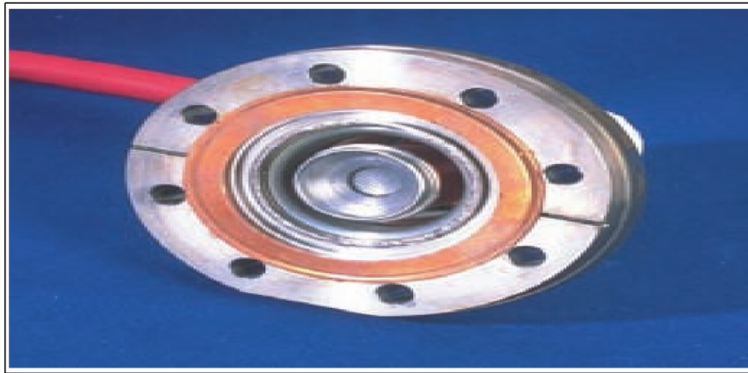
FIGURE 1.6: Removable electron triode gun for a typical high energy linac [37].
