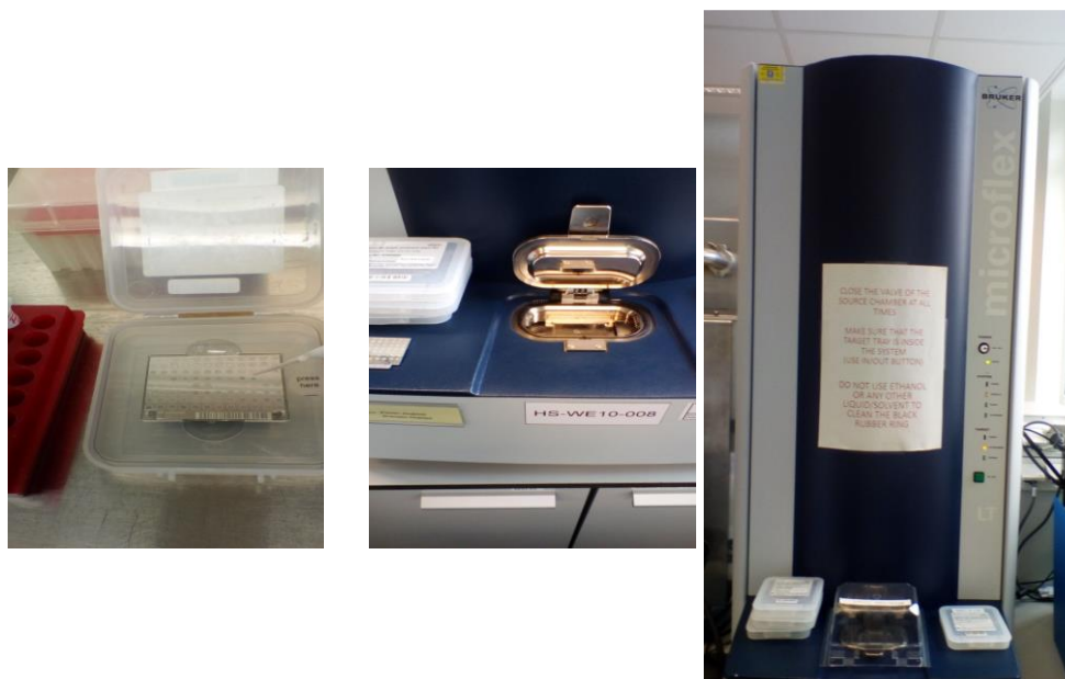
Figure 12: Photo of MALDI-TOF Mass Spectrometry unit used at LMG Lab, Ghent University
