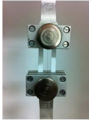
Figure 1.19: Photograph of the Zwick Z2.5 traction device. [46]
