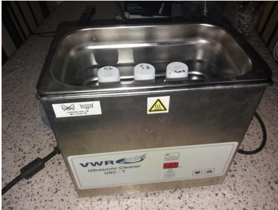
Figure 2. 13: Three nanofluids with volume fraction 0.0025%, 0.005% and 0.01% exposed in Ultrasound for 30 minutes.
