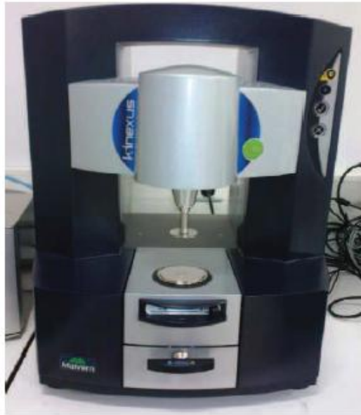
Figure 3.4: Kinexus Malvern rotary rheometer
