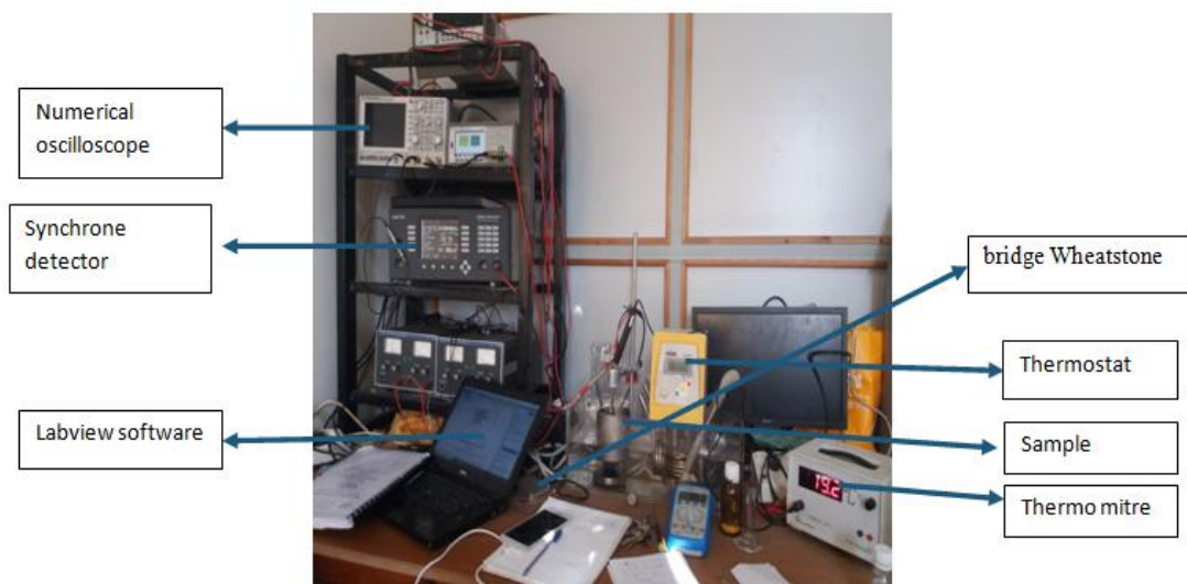
Figure 2. 14: Measurement bench instrumented with Labview software
