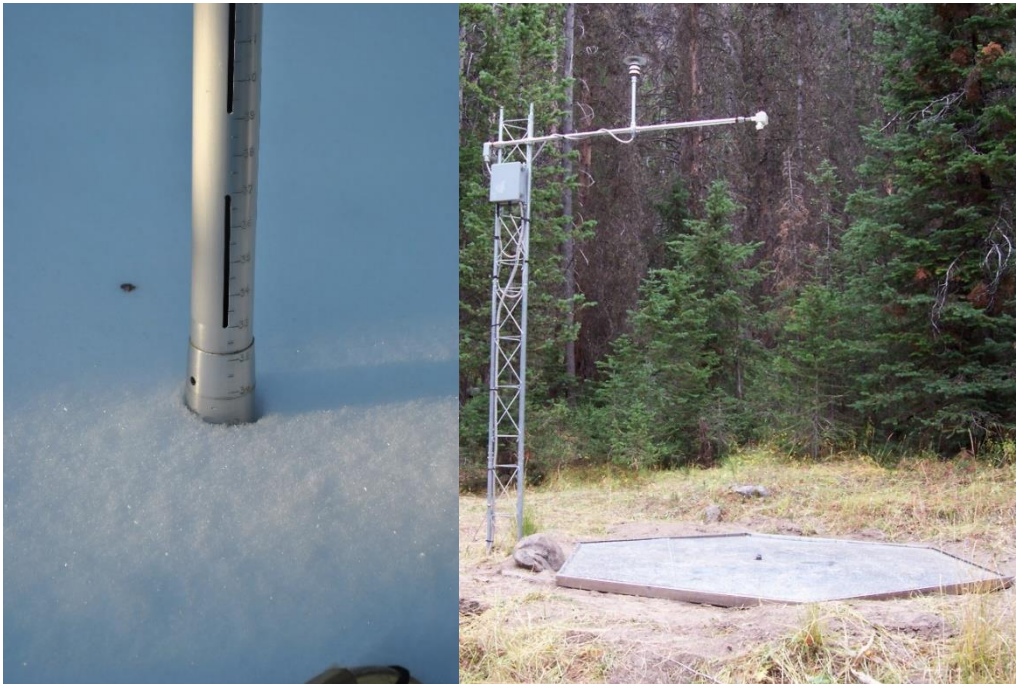
Figure 5. Left: snow depth sampler. Right: measurement station holding an ultrasonic snow depth sensor (source: https://www.nrcs.usda.gov/ ).
