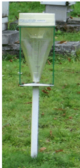
Figure 3. Funnel-shaped manual RG (source: https://the-weather-station.com/ ).
