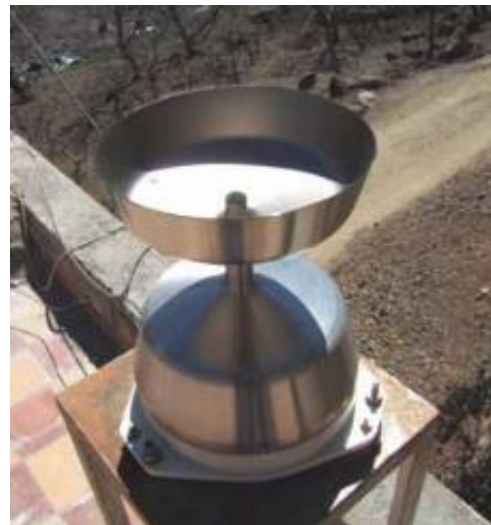
B- Tipping bucket rain gauge
