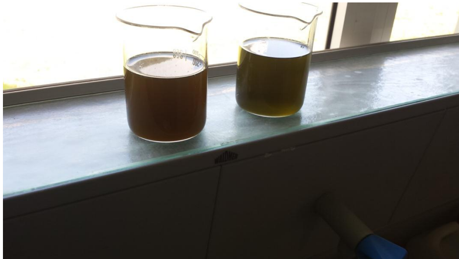
Figure 4: Phosphoric acid clarified 54% in P 2 O 5 , from the Jorf-Lasfar platform (beaker on the left) Phosphoric acid purified 54 % in P 2 O 5 , from the Safi platform (beaker on the right)
