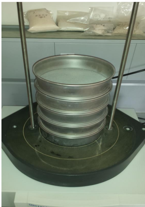
Figure 3: Vibration Tammy to adjust the solid phosphate samples to the desired particle size distribution.
