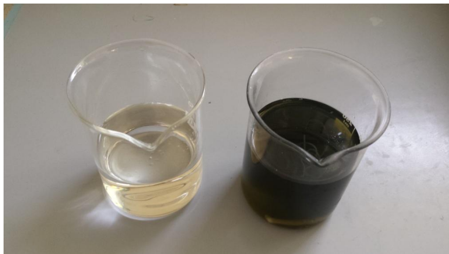
Figure 3: Phosphoric acid clarified 54% in P_2O_5 , Density: 1608 g/l (beaker on the left) Phosphoric acid purified 61% in P_2O_5 , Density: 1720 g/l (beaker on the right)
