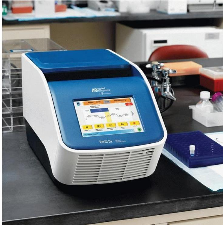
**Figure 16 : Appareil Veriti® 96 well Thermal cycler, Applied Biosystems**
