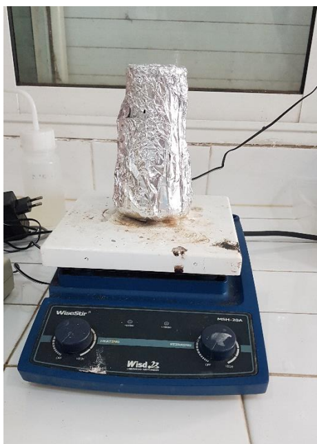
Figure 15: Extraction of secondary metabolites on a magnetic stirrer in dark conditions
