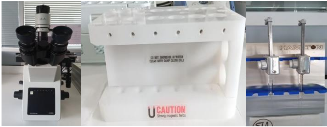
figure 13: a). inverted fluorescence microscope used to adjust the concentration and read the results. b) magnet with a strong magnetic fields for T lymphocyte-beads isolation. c) tissue typing syringes
