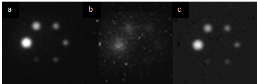
Figure 4.22: The reconstructed images of simulated Jaszczak; (a) without the TEW image, (b) Scatter image, (c) with the TEW image.
