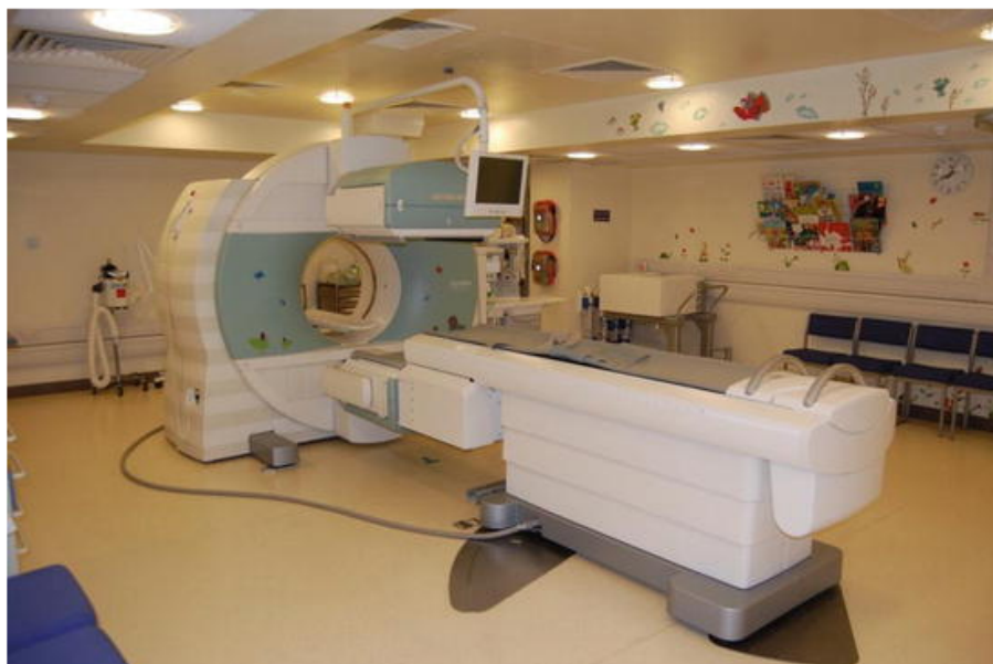
Figure 1.1: Siemens Symbia T2 SPECT CT gamma camera
