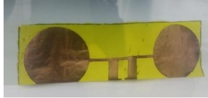
Figure 79: Prototype of the Proposed Flexible Tag Antenna
