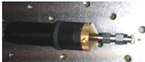
Figure 56: LXMS31ACNA-01 Chip Connected by SMA Connector
