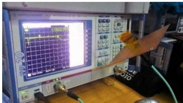
Figure 81: Measurement Set-Up Using Rohde & Schwarz ZVB 20 VNA
