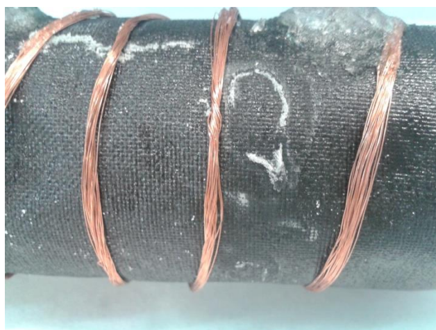
Fig 8: Salt formation on the membrane assembly during and after treatment
