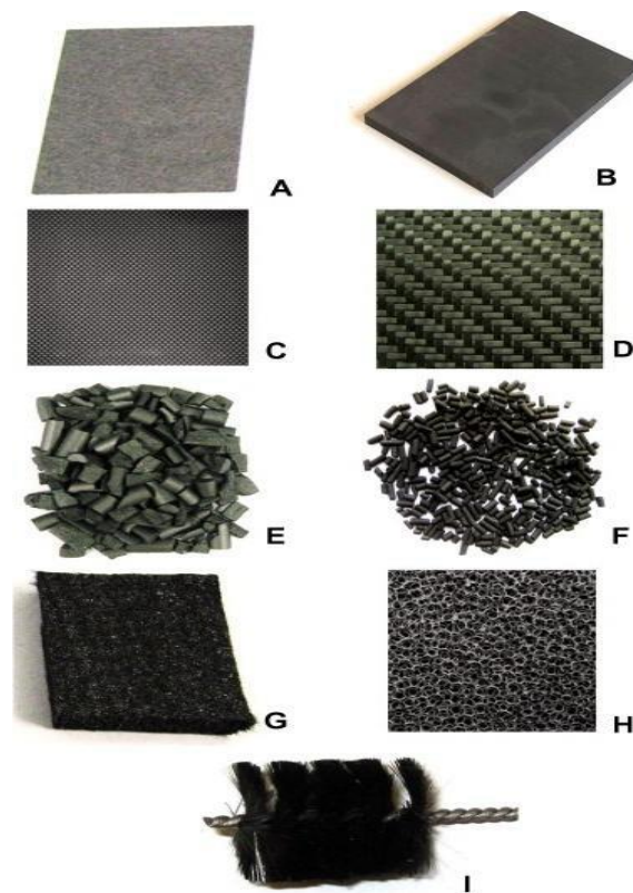
Fig 4: Photos of anode materials used in MFC: (A) graphite paper, (B) graphite plate, (C) carbon fabric, (D) carbon mesh, (e) granular graphite, (F) activated carbon granular, (G) carbon felt, (H) crosslinked vitreous carbon, (I) carbon fiber brush
