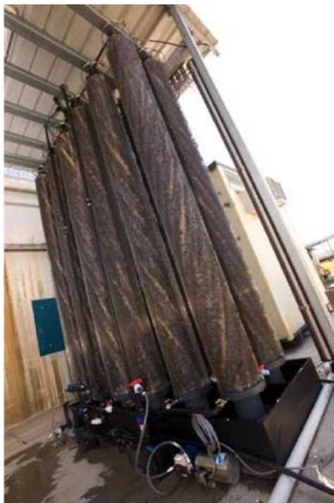
Fig 12: Applications for MFCs. (A) Pilot-scale microbial fuel cell constructed by the advanced water management centre at the University of Queensland and Foster's brewery in Yatala, both in Australia
