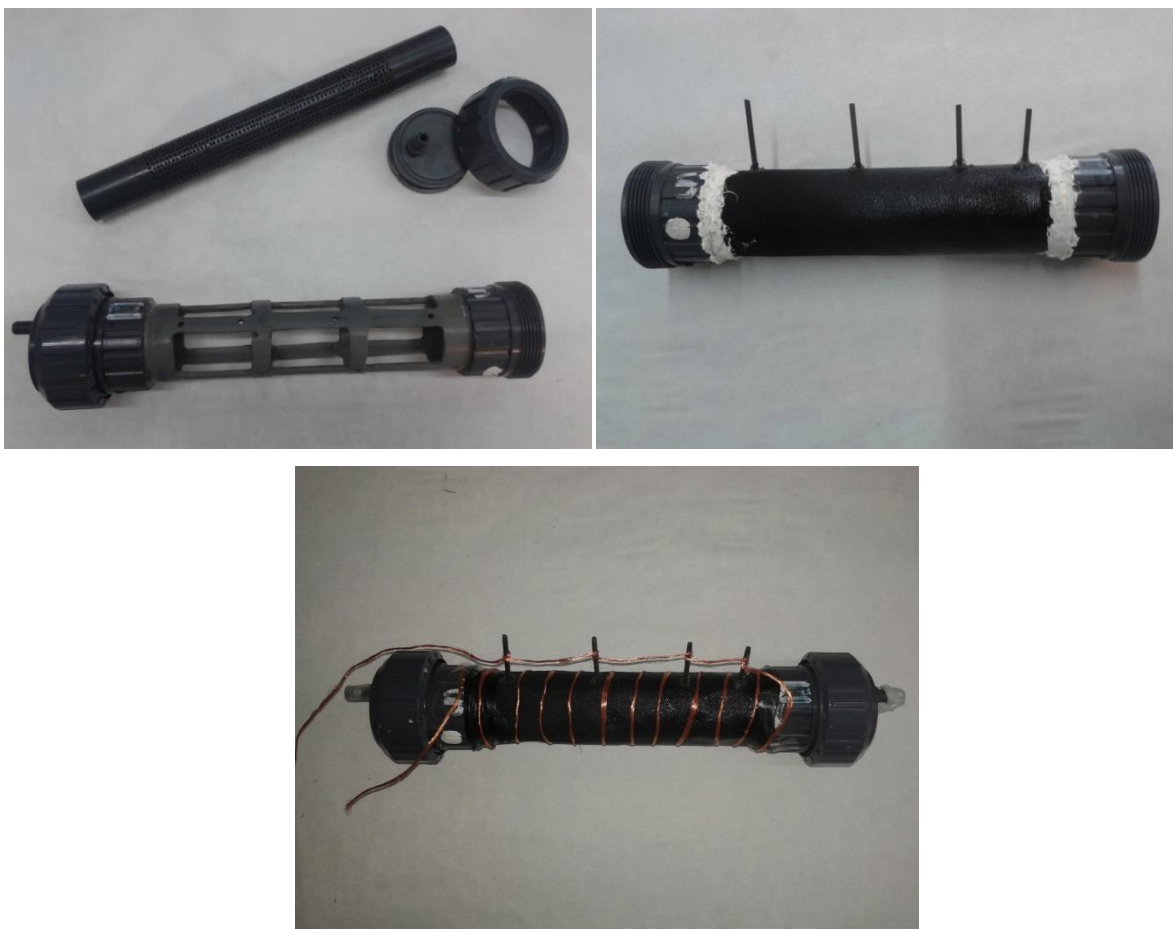
Fig3: Components of the horizontal reactor, embedded membrane-cathode assembly and the final design of the single-chamber air-cathode microbial fuel cell
