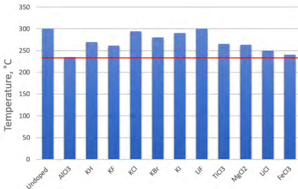
FIGURE 1.9: The desorption temperature as function of each additive
