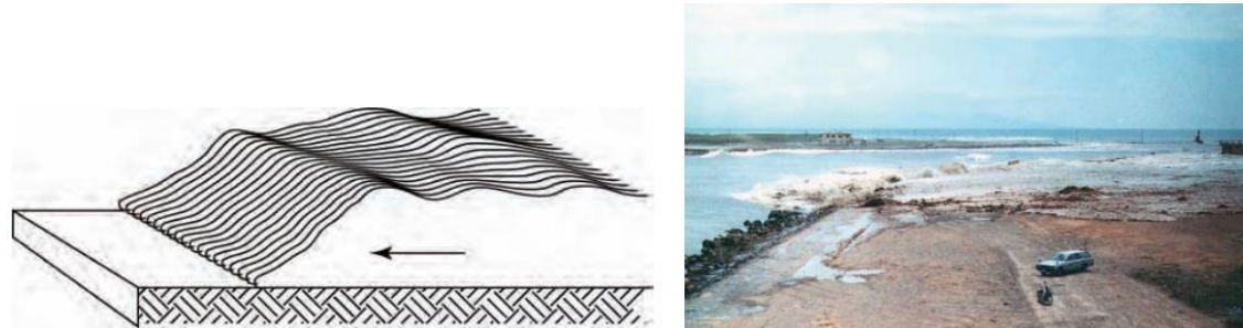
Figure 19: surge form when tsunami rush up on shore (after FEMA P646)
