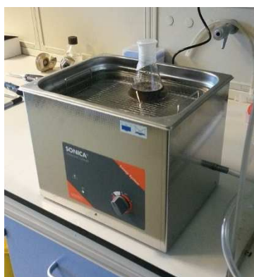
Fig 33. Image representation of the experimental setup used for ultrasonic assisted extraction.
